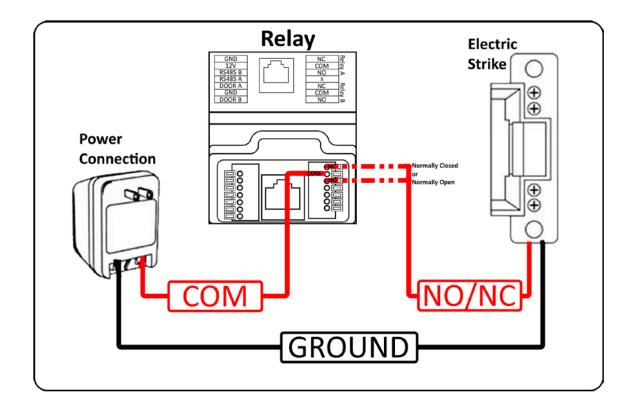
NC – COM if your Door Strike type is unlocked when power off and locked when power on.NO – COM if your Door Strike type is unlocked when power on and locked when power off.
