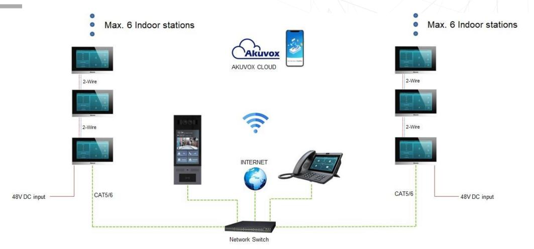
If you can connect first indoor monitor to Network directly via CAT cable, you don't need to use NS-2 for buildings. You can refer this diagram.
