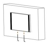
Use Allen wrench fix two M2x5 hex socket screws into the bottom of the device. And the installation is done.
