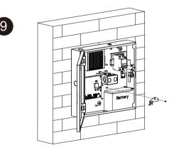
Place the battery as shown in the figure, and use the fixing plate and M3X5 crohsshead screw to fix it.
