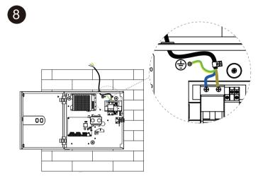
Connect the provided wire as shown in the figure, then use M3X5 crosshead screw and wire fastener to fix the wire on the A094.
