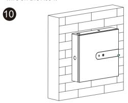
The installation is done, and please lock the cover. Then remove the protective film.
