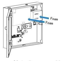
Open the cover of device, then remove and throw out the protective foams of power supply and air switch.
