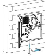
Knock a lead hole with the appropriate tool according to the desired wiring position.
