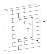
Insert plastic wall anchors into the holes.
