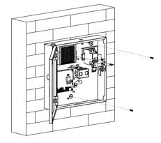
Fix A094 with three ST4x20 crosshead screws on the wall.
