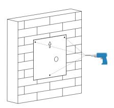
Stick the wall-mounting template on the wall where the device needs to be installed. According to the screw hole position on the template, use an electric drill to drill the hole with a diameter of 6mm and a depth of 25mm.
