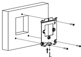
Drive the set screw in to hole in the bottom center of the bracket using Allen wrench attached and make sure that the tail-end of the screw is flushed with the hole surface of the bracket, then fix the bracket on to the wall using three ST4x20 screws.
