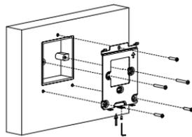
Drive the set screws in to hole in the bottom center of the bracket using Allen wrench attached and make sure that the tail-end of the screws is flushed with the hole surface of the bracket, then fix the bracket on to the wall using three ST4x20 screws and two M4x30 screws.
