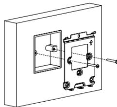
Take off the M4x30 screws along with the wall bracket.
