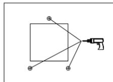
Take off the bracket and drill the three marked fixing holes on the wall. ( 5 mm in diameter and 25mm in depth)
