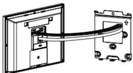
Connect the network cable and signal cable to their corresponding interfaces at the back of the device.
