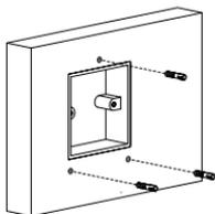
Insert the plastic wall anchors in to the three drilled holes.
