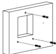
Insert the plastic wall anchors attached in to the fixing holes.
