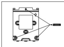
Centre align the square hole of the wall bracket and the hole on the wall, and then mark the three fixing holes of the bracket on the wall.
