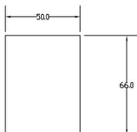
According to the position of the cable in the wall, cut a square hole (height\*width\*depth= 66 mm\*50 mm\*55 mm)in the wall used to accommodate all the cables.
