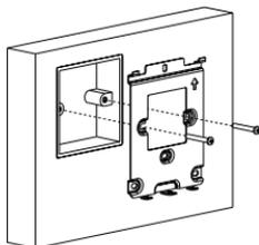
Fix the wall bracket on to the injunction box using two M4x30 screws.
