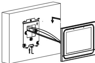
Hang the device on to the square hooks on the wall bracket using the two square holes at the back top of the device, and keep the device parallel to the wall before tightening the the bracket using the M3 set screw.
