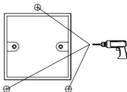
Drill three holes on the marked hole positions. (5 mm in diameter and 25 mm in depth)
