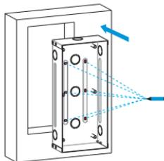
Insert the embedded box into the hole and make sure the cables of the device can route through the cable hole. Then mark the six holes of the wall embedded box on the wall.
