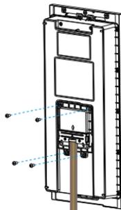
For convenient wiring, hang R27X on the wall-mounting box/ flush-mounting bracket with rope. Then insert the silicon rubber sealing ring into the groove.
