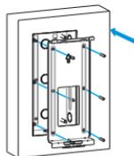
Dig out a square hole (height\*width\*depth=262.5\*121\*60 mm).
