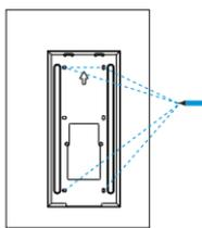
Mark the four holes of the wall-mounting box on the wall.
