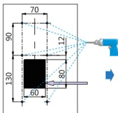
Use a hand drill with 5 mm diameter bit to make the hole in marked positions. Dig out a square hole.(height\*width\*depth=80\*60\*50 mm)
