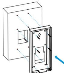
Fix the wall-mounting box with six ST4x20 screws.
