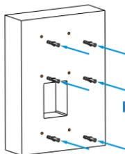
Insert the plastic wall anchor into the holes you drilled before.
