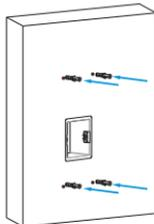
Insert the plastic wall anchor into the holes.
