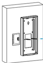
Fix the wall-mounting box on 86 embedded box with two M4x30 screws.
