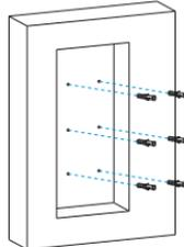
Insert the plastic wall anchor in the hole you drill before.
