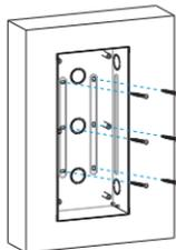
Place the embedded box into the square hole until the edges of which align to the wall and make all cables go through the cable hole. Fix the embedded box with six ST4x20 screws.
