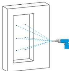
Take down the embedded box, then use a hand drill with 5mm diameter bit to make holes in the marked positions.
