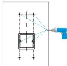
Use a hand drill with 5mm diameter bit to make holes in the marked positions.
