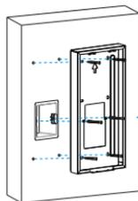
Fix the wall-mounting box with four ST4x20 screws and two M4x30 screws.
