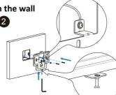
Twist M3x10.5 screw into the bottom hole of the wall bracket until the tail of which align to the edge. Then fix the wall bracket on the wall with two/four M4x30 screws. If there is a ground wire to be connected, use M3x6 screw to fix it on the wall bracket
