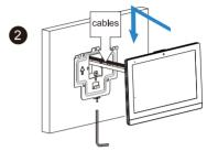
Push down to fix the device securely. Use the Allen wrench to tighten the device with one M3x10.5 screw.
