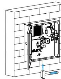
Knock a lead hole with the appropriate tool according to the desired wiring position.
