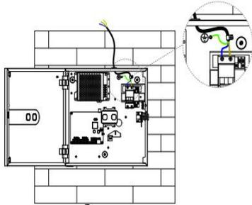
Connect the provided wire as shown in the figure, then use M3X5 crosshead screw and wire fastener to fix the wire on the A092.
