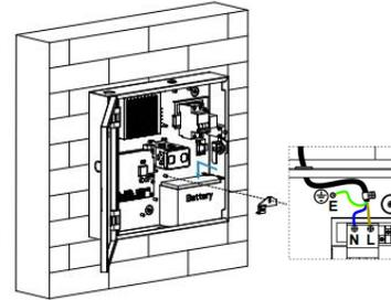
Place the battery as shown in the figure, and use the fixing plate and M3X5 crosshead screw to fix it.
