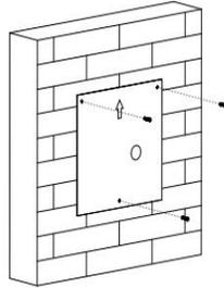
Insert plastic wall anchors into the holes.
