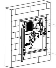
Fix A092 with three ST4x20 crosshead screws on the wall.
