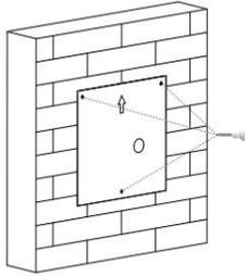
Stick the wall-mounting template on the wall where the device needs to be installed. According to the screw hole position on the template, use an electric drill to drill the hole with a diameter of 6mm and a depth of 25mm.
